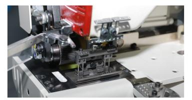
AGM Special KM 930 SDX-T3 model automatic without feed dog waistband attaching machine designed for jeans trousers, chino type casual trousers, jeans jackets and work wear manufacturers.
