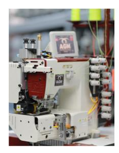
Allows to attaching wider waistband forms gauge set between minimum 1 3/4" - maximum 2 3/4"
