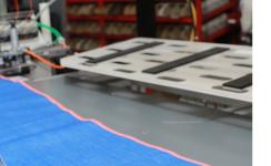
New designed adjustable accurate zyppy unit that moves left- right and up-down according to different kinds of fabrics(light to heavy fabrics included full lycra and power stretches).
