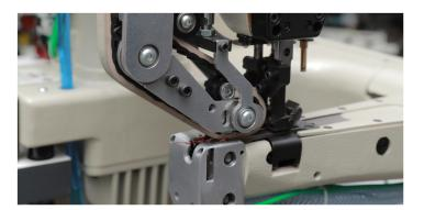
This machine is the result of AGM Special R&D team's long-lasting effort. Equipped with a special full-oil gearbox system and special movable 3 roller pallet puller system, this machine will minimize the stitch defects usually seen in seam joint areas and during long operations.
