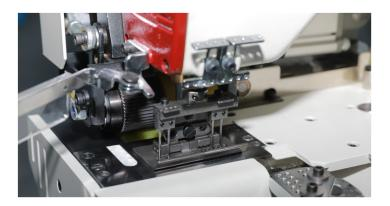
Electronic waistband attaching sewing machine specially designed for attaching LEVI'S type waistbands.
