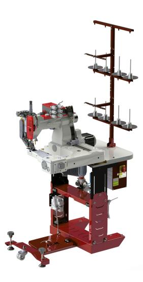
Stand-alone adjustable differential feeding system that provides ease of use for the operator and allows perfect sewing of different fabrics.
