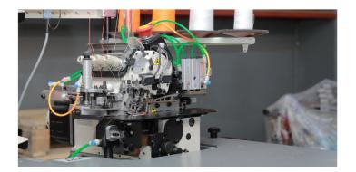
Unique design that allows left and right two panels of the jeans trousers to be feeding from top to bottom at the same time.
