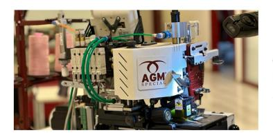
KM 921 AR-T3 model waistband attaching/sewing automat is a flexible, effiency and high quality output. The daily capacity is 1700-2500 pcs/8 hours. The innovative transport system allows the machine to perform on all type of fabrics.
