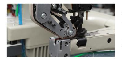
This new machine is the result of AGM Special R&D team's long-lasting effort. Equipped with a special full-oil gearbox system and special movable 3 roller pallet puller system, this machine will minimize the stitch defects usually seen in seam joint areas and during long operations.
