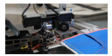
The paradigm-shifting innovation. The world's first and only double-head serging automat. A real game changer resulted from many years of effort by Agm Special engineers. Innovative and practical, this serging machine can sew simultaneously both right and left trouser panels. The KLR 400-T2 is economically viable because it reduces by half the number of operators previously required for the this type operation.
