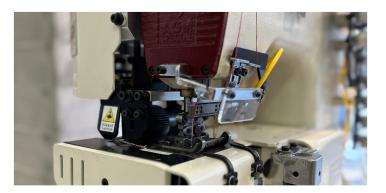
The World's first and only Hybrid Waistband Attaching/Sewing Automat. This machine can be used for attaching both standard straight and curved waistband forms and also suitable piece by piece waistband attaching/sewing method(LEVI'S type). The transformation is simply done by changing the proper gauge set and LEVI'S type apparatus.
