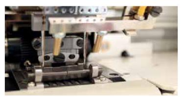
SPECIAL DESIGN PRESSURE FOOT AND FEED DOG Special designed pressure foot and feed dog for LEVI'S type waistband attaching method by AGM Special.
